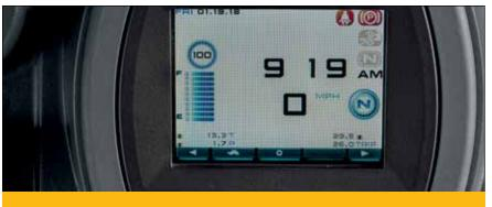
The display includes date, clock, speedometer, vehicle hour meter, warning icons and more.
